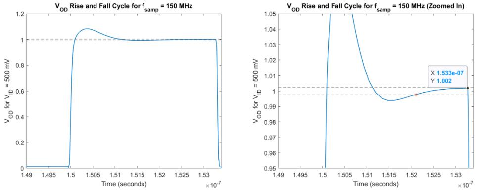
Figures 5 and 6: Measurement of dynamic settling error using the original sampling frequency of 150 MHz; convergence of output error within 0.25% is shown at the red asterisk
