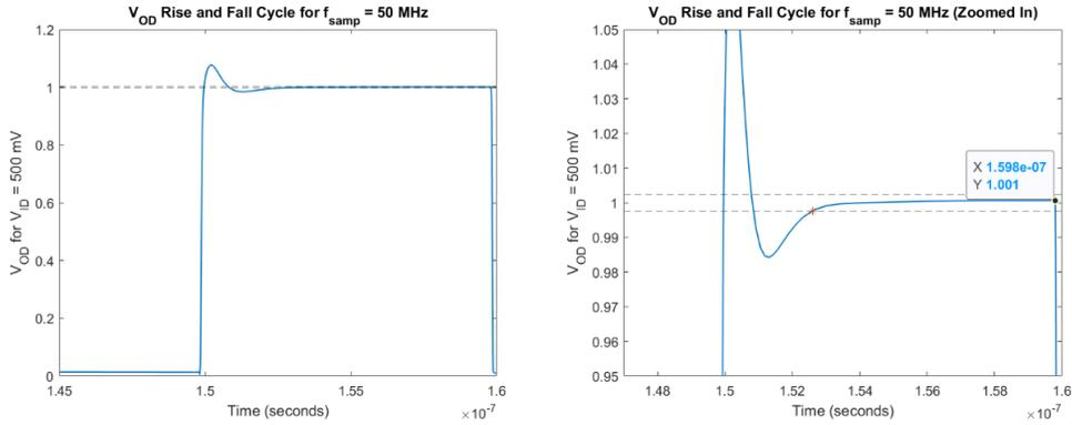
Figures 3 and 4: Measurement of static settling error using a sampling frequency of 50 MHz; convergence of output error within 0.25% is shown at the red asterisk
