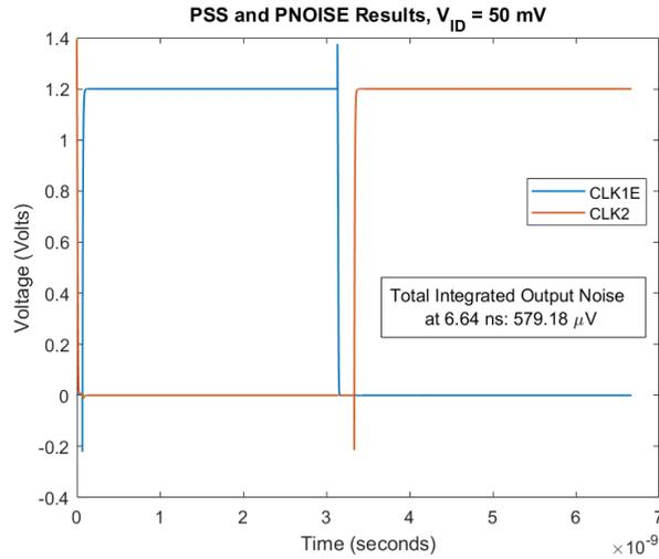
Figure 7: Periodic steady-state (PSS) and periodic noise (PNOISE) simulation results, with rms total integrated output noise near the end of the evaluation phase
