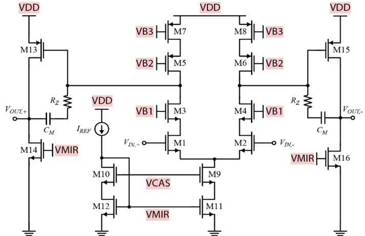
Figure 2: Schematic of OTA, numerical values for all components and biases and provided in Tables 2 and 3; note that VMIR is set by the wide-swing diode connection of M12, rather than by an external voltage.
