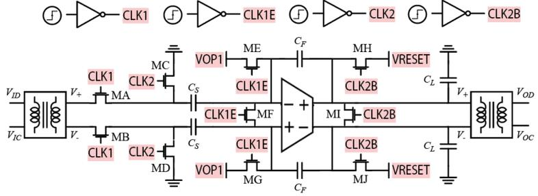
Figure 1: Selected SC topology, with buffered clock generation from ideal pulse voltage sources indicated at the top
